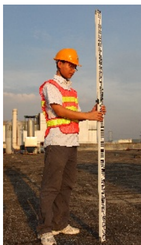
ACS5 5m Aluminum Code Staff FCS2 2m Fiberglass Code Staff, two section
